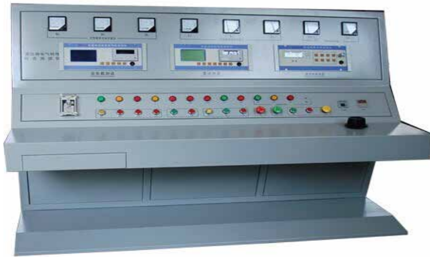
Comprehensive test platform for power transformer
