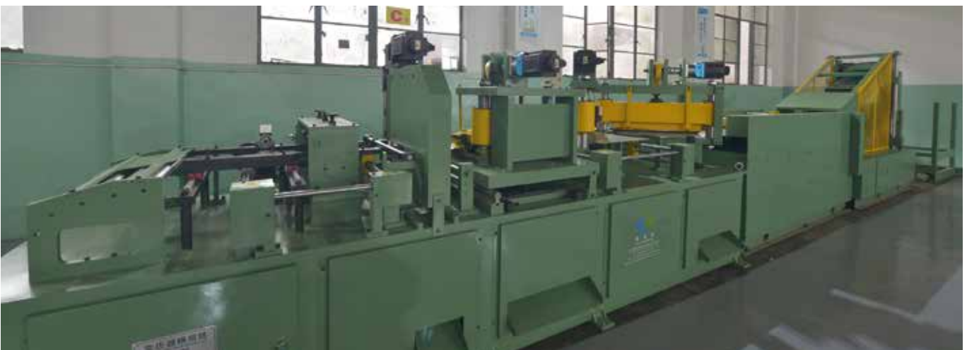
Silicon steel sheet crosscutting machine
