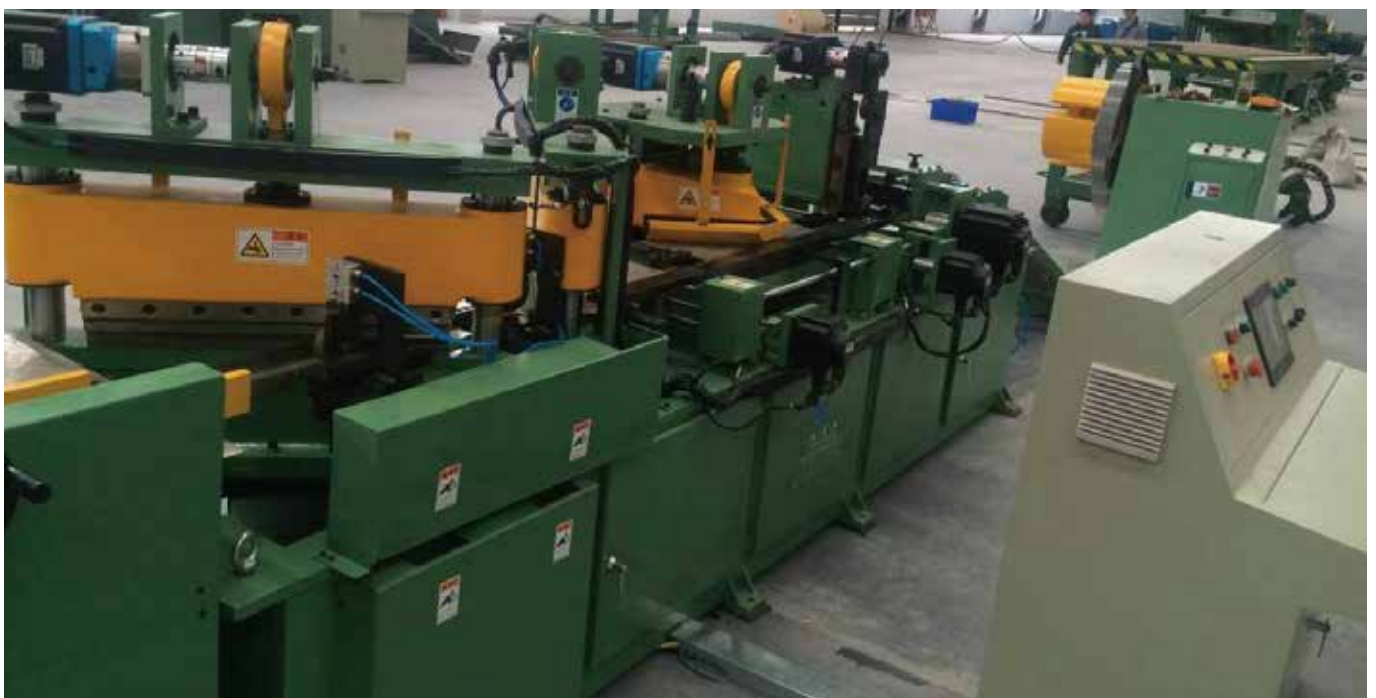
Silicon steel sheet crosscutting machine
